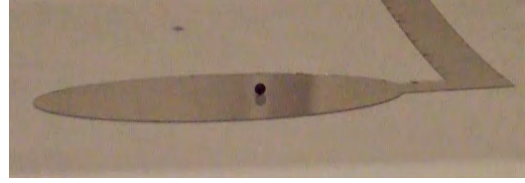
Figure 8. An expanded polystyrene bead of 2 mm diameter was attached on the electrode to evaluate the mechanical response experimentally.
