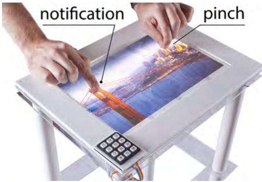
Figure 4. (Background removed) A user is exploring tall buildings by pinching and pulling the display with one hand, and simultaneously receiving peripheral visual and tactile notification at the other hand.
