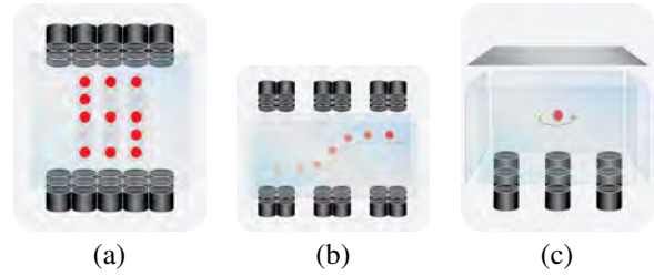
Figure 6. (a) A bistable display with tightly packed transducers and dedicated electrodes. (b) A 3D game with user-defined configuration of transducers and two electrodes for flipping the voxel. (c) Four electrodes for rotating a voxel, which is levitated using a reflector.
